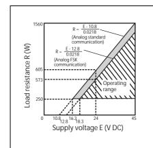
Figure 1 Supply voltage vs. load resistance characteristics
