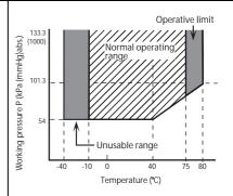
Figure 3 Working pressure and temperature of wetted parts section for oxygen and chlorine service
